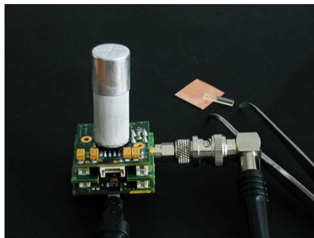
Fig. 1: LYSO based scintillator coupled to a SiPM in the capsule and mounted on a fast low-noise trans-impedance amplifier board.
